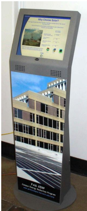
17" Touchscreen kiosk in lobby of the Harvard Science Center. This unit includes dual screen and custom detail on the front.
